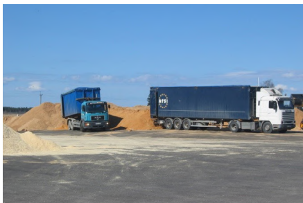
Figure 5.11. Transport of wood chips by container truck or special truck adapted for the transport of wood chips, (photo P. Muiste)
