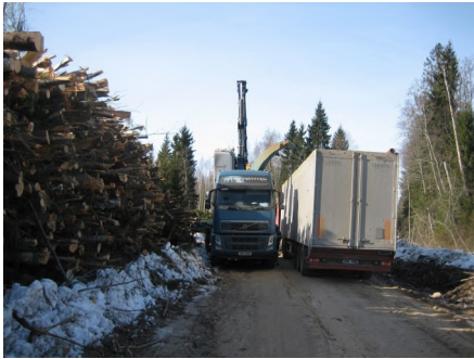
Figure 5.9. Chipping of logging residues into a truck bed, (photo P. Muiste)
