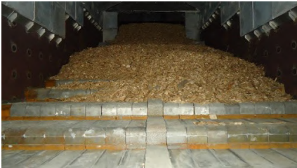
Figure 7.2. Moving grate for burning wood fuel [40, 41]
