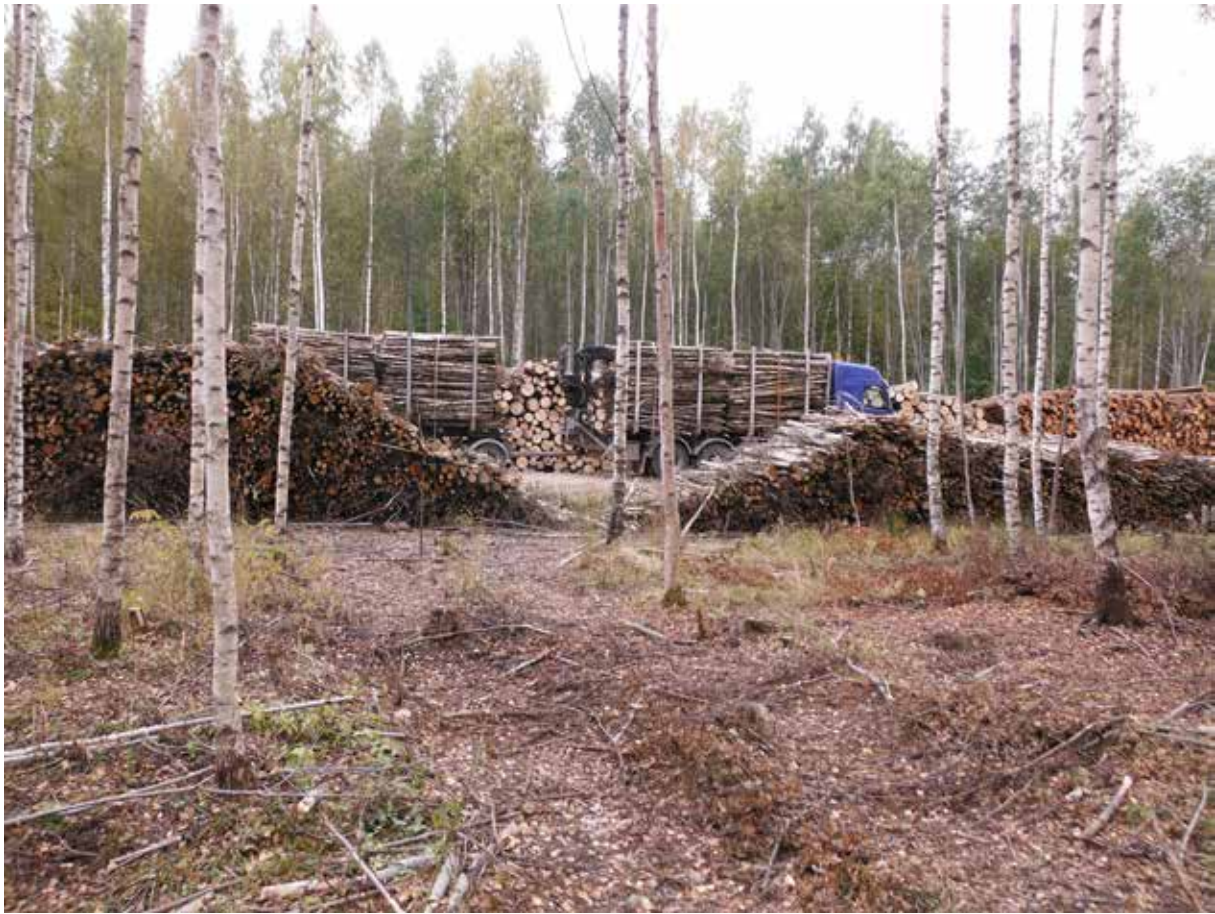
Picture 17. Depending on how well delimbed the material is, it can possibly be run on ordinary timber trucks. Biofuel produced from small sized trees in pre-commercial thinnings of birch stands is delivered to a pellet factory in Jēkabpils city, Latvia. (Photo: Andis Lazdiņš)
