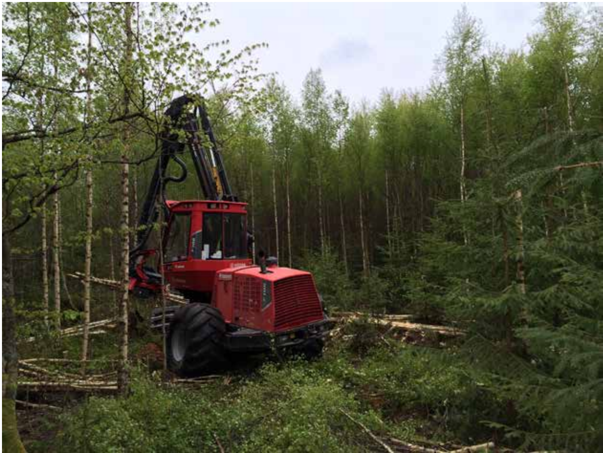
Picture 13. Much of the harvester's time in stands of small trees is spent on crane operation. Birches are removed and spruces are left. (Picture: Örjan Grönlund)
