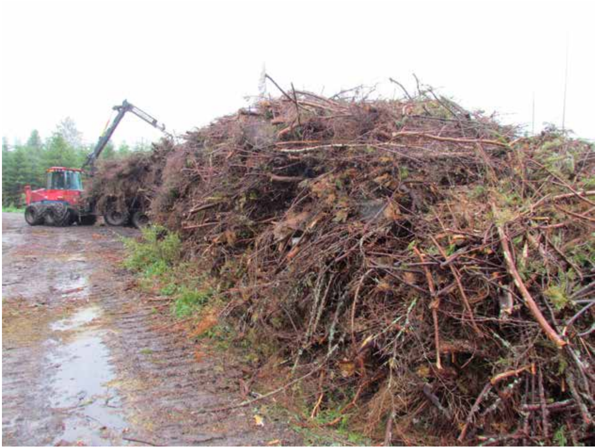
Picture 20. The major part of forest chips are produced at the roadside storage sites – here the unloading and piling of logging residues is ongoing. (Photo: Lars Eliasson)
