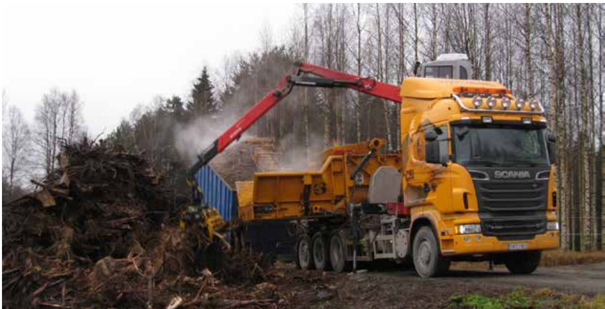
Picture 42. Stumps are crushed at an appropriate location before deliveries to energy plants. (Photo: Juha Laitila)
