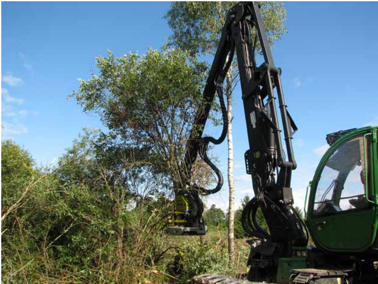
Picture 47. In the Baltic Countries, as result of the land use history a lot of naturally regenerated broadleaved stands are growing on old agricultural fields. Extraction of biofuel in abandoned overgrown farmlands with a felling head in central Latvia. (Photo: Andis Lazdiņš)
