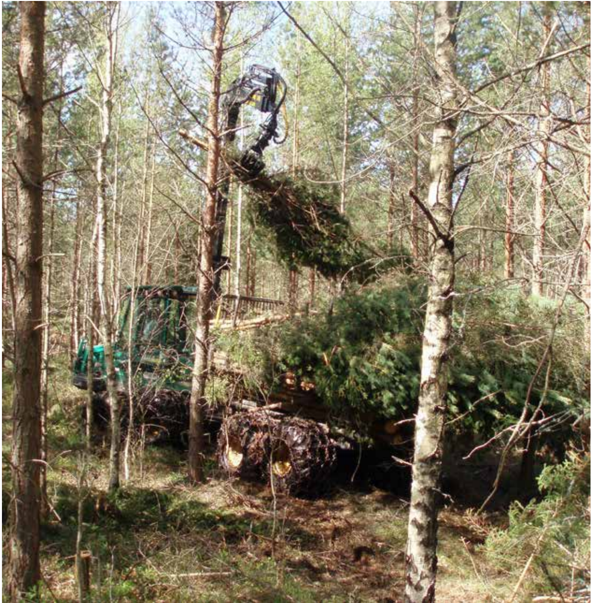
Picture 15. The slightly lower payload is due to greater air content in load because of the branches and very small-dimensioned wood. (Photo: Maria Iwarsson Wide)
