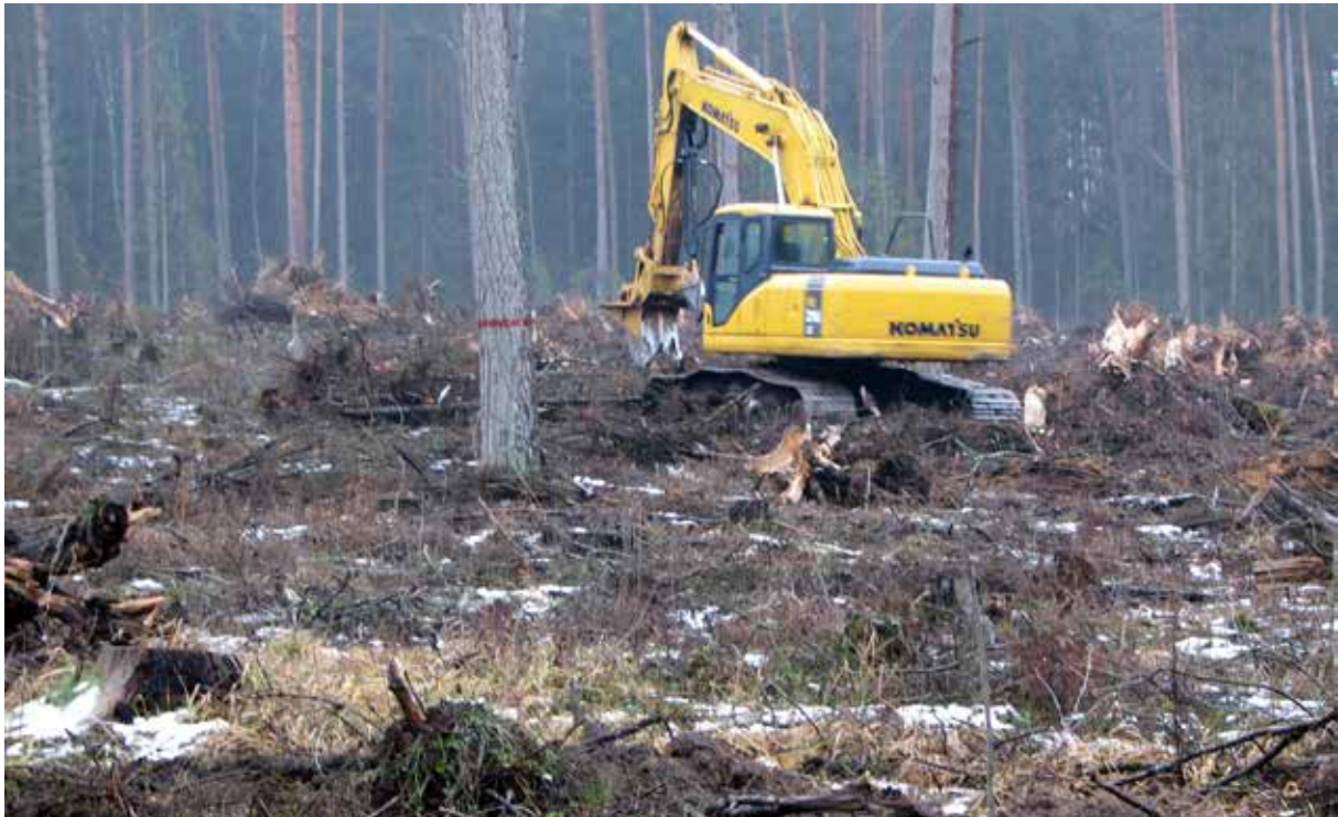
Picture 38. The stumps are lifted, split and collected into piles with excavators equipped with a special device for the specific operations. Stump extraction after the regenerative felling of spruce stands was one of the first stump extraction trials in Latvia. (Photo: Valentīns Lazdāns)
