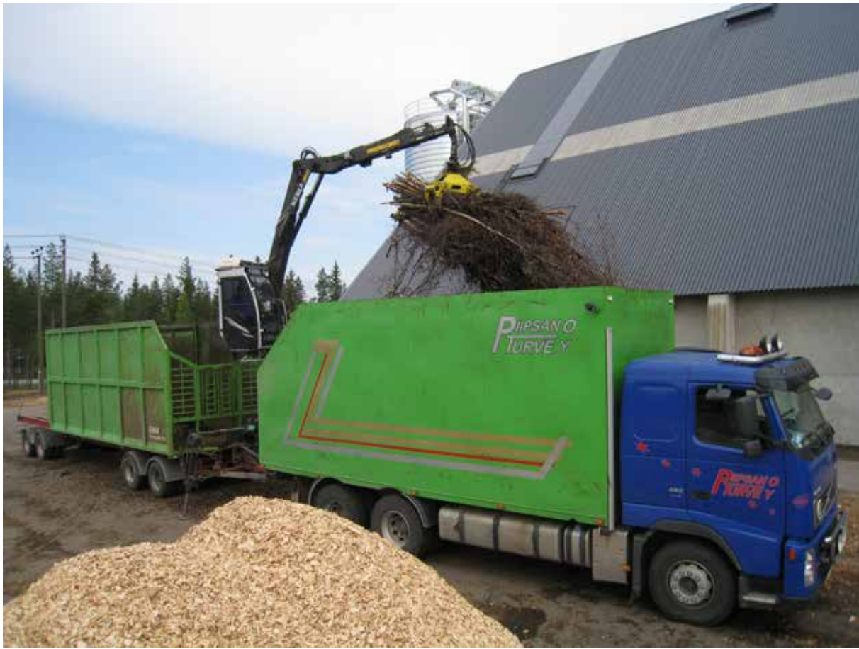
Picture 18. Undelimited energy wood or loose logging residues can be transported to a terminal or end-users on biomass trucks with covered sides and bottom. (Photo: Juha Laitila)
