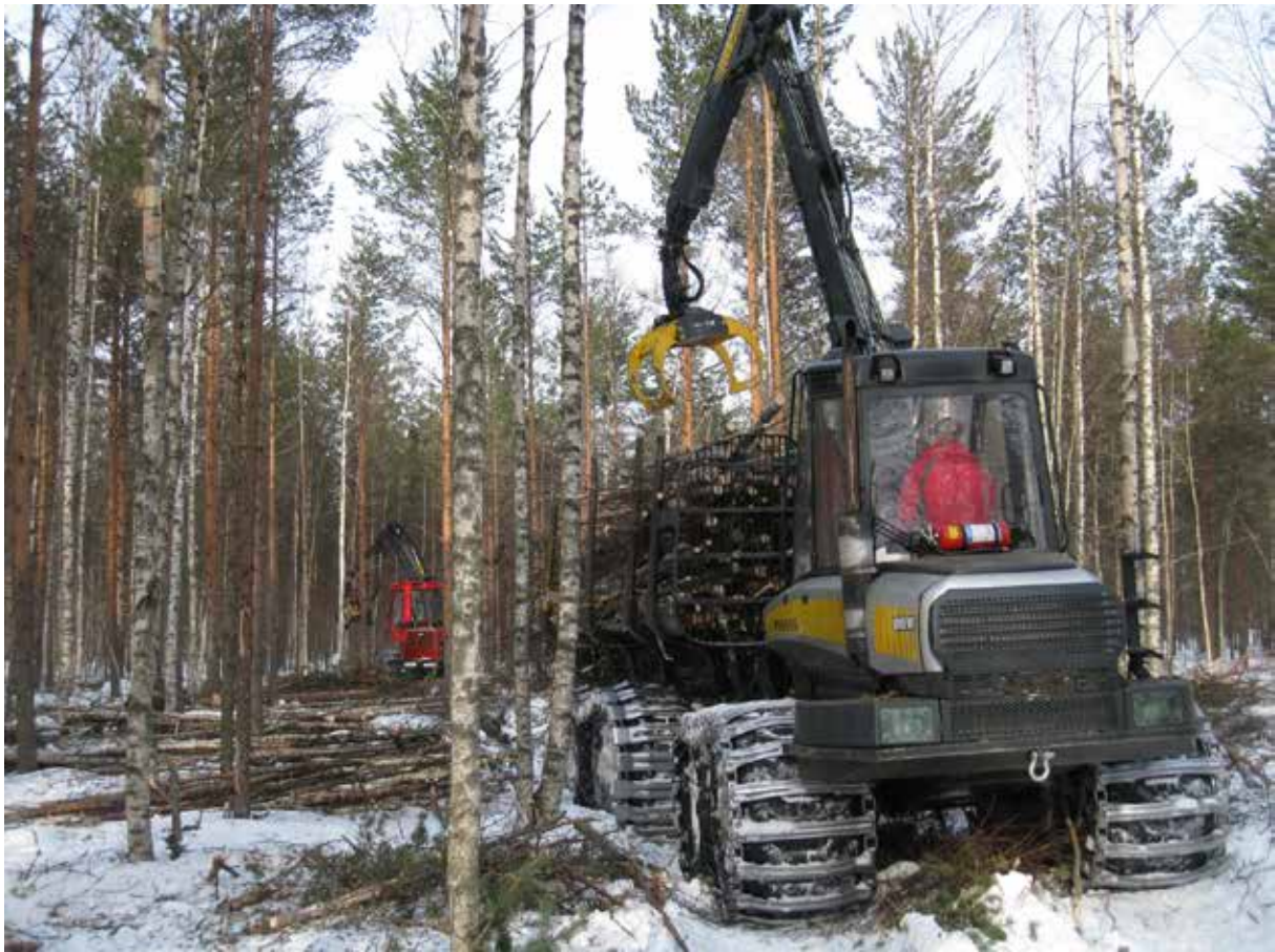
Picture 12. The traditional two-machine method – with a harvester for felling and cutting, and a forwarder for short distance transportation to the forest site storage location. (Photo: Juha Laitila)
