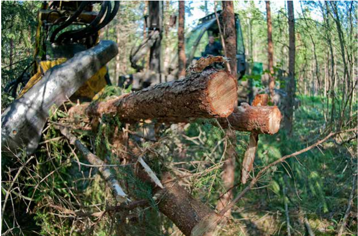
Picture 6. Logging operations are done with a harvester equipped with grapple to be able to handle multiple stems at a time. (Photo: Erik Viklund)
