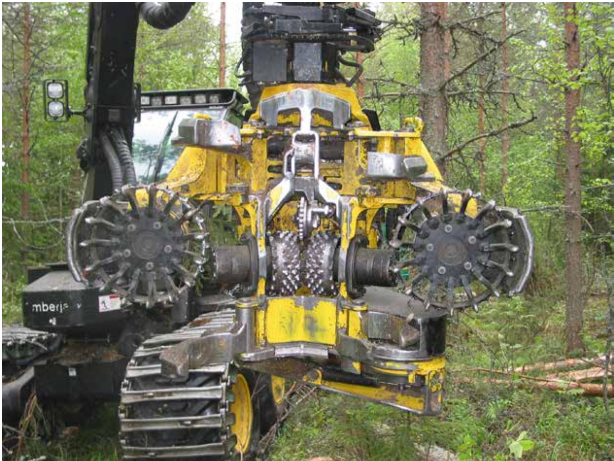
Picture 14. It is quick to switch between harvesting pulpwood and forest fuel with an accumulating harvester head equipped with feed rollers. (Photo: Juha Laitila)
