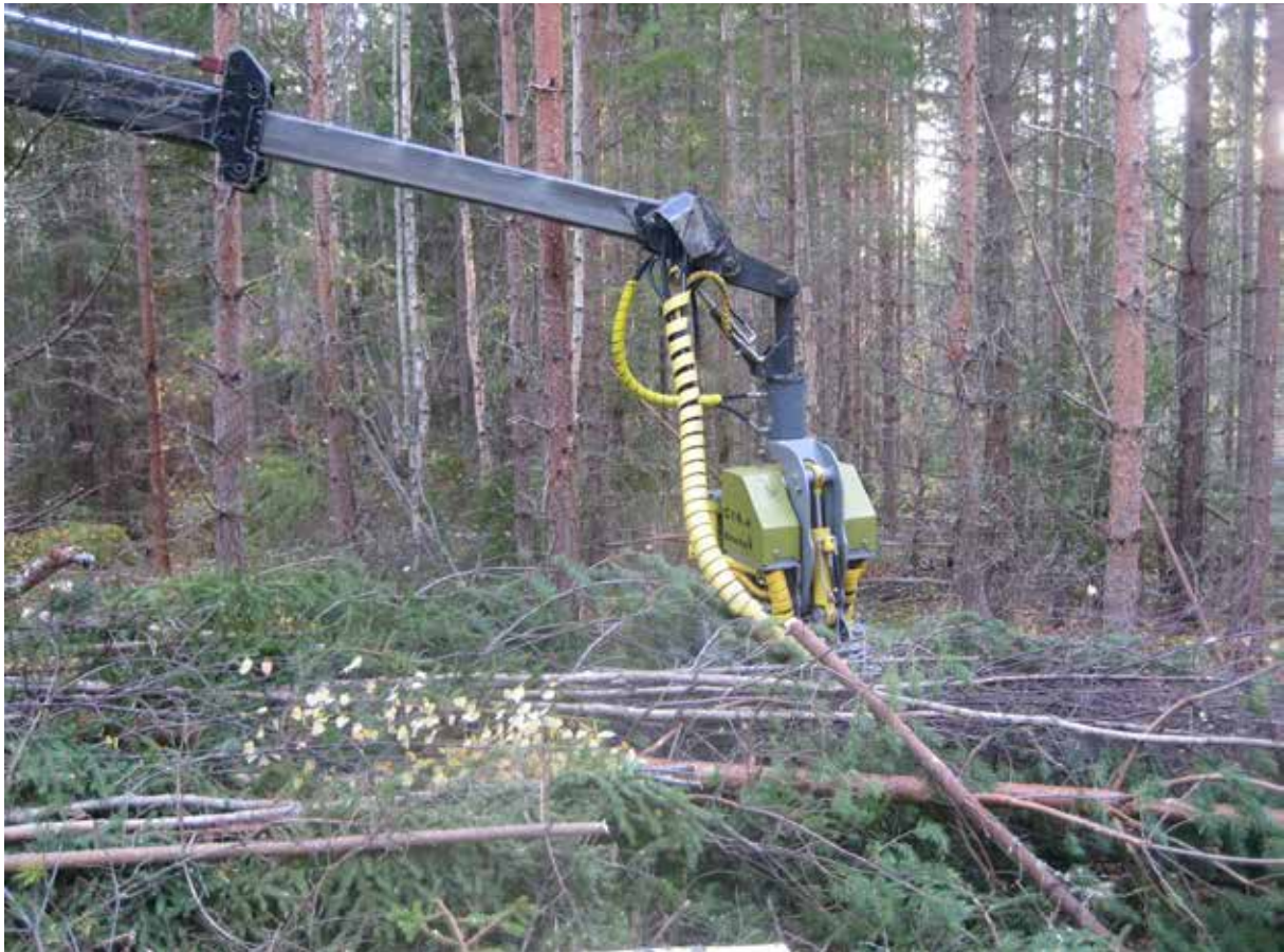
Picture 8. Three technical cross-cutting solutions are used for felling small trees with a harvesting head. (Photo: Maria Iwarsson Wide)
