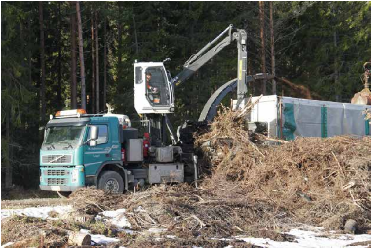
Picture 10. Storage and chipping takes place at the roadside, and the chips are then transported directly, or via a terminal, to the customer. (Photo: Lars Eliasson)
